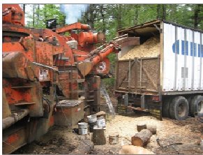
Chipper on log landing.
